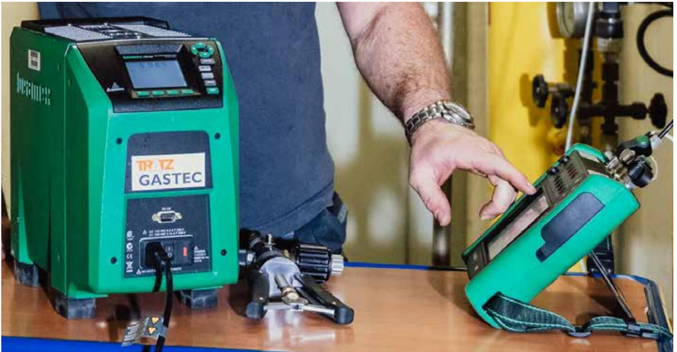
Another Tratz Gastec division focuses on gas pressure regulator maintenance, functional tests, and visual checks. A database is under development at this division to store the data generated by these processes. The Beamex CMX calibration management software and the Beamex bMobile calibration application play an important role here. Checklists created in CMX can be ticked off at the customer's site via the bMobile app. This makes it easier
